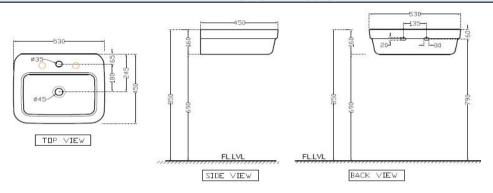
ALL DIMENSIONS ARE IN MM. (TOLERANCE ± 5 MM)
